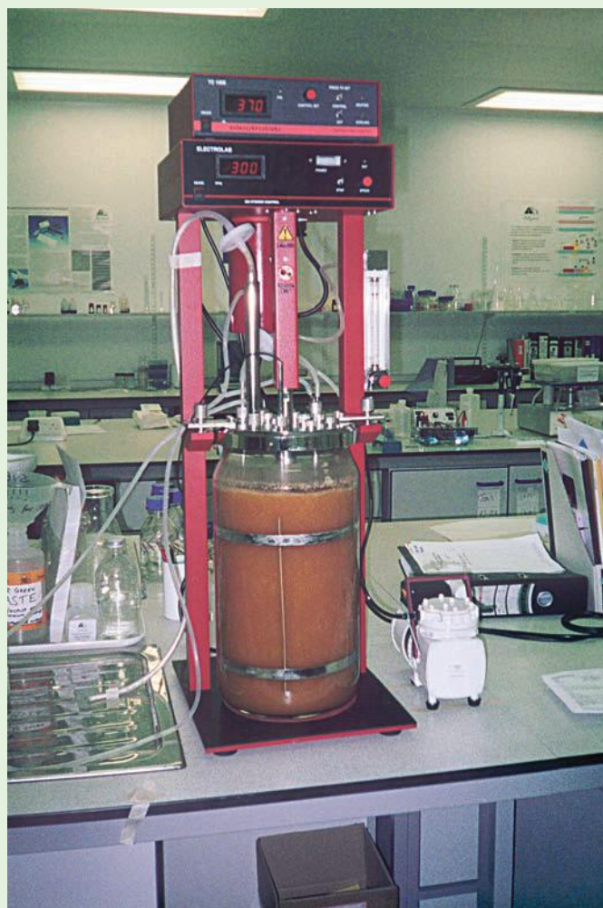
Figure 20.3 A laboratory fermenter for antibiotic production, which will eventually be scaled up to 10000-litre fermentation vessels.
